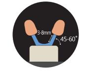
Connect the object and investment ring base at an  $\angle 45$ ~60° angle, at a length of 3~8mm, using  $\emptyset$ 3~3.5 mm of sprueing wax.
